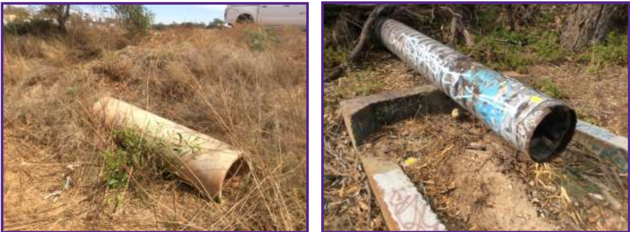
Figure 4.1: Common asbestos pipes found at Water Corporation (left image - AC Pipe Exterior of Compound in Karratha, right image – asbestos bitumen coated pipe in Karrinyup
