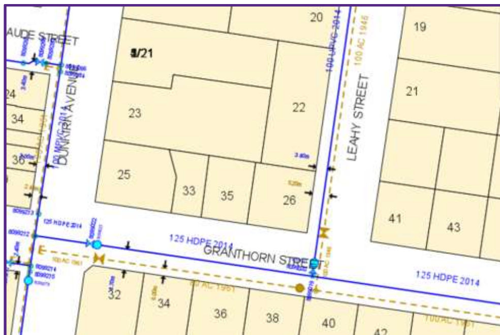
Figure 1.4: An example of a GIS snapshot of a replaced water main (note the blue line is the replacement main, and the gold/brown dotted line is the old AC main)
