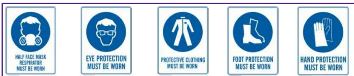
Figure 5.2: PPE that employees and contractors must wear when cutting or in the vicinity of cutting asbestos pipes (including the special requirements)
