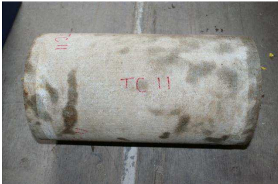
(a) 300 mm sub-sample for crush test
