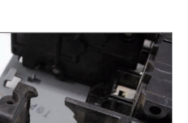
FIGURE 10 - THE DAMAGE TO THE INSULATING STRUCTURE OF THE PANEL (FIG. 8) IS MORE CLEARLY VISIBLE WITH THE BREAKER REMOVED.
