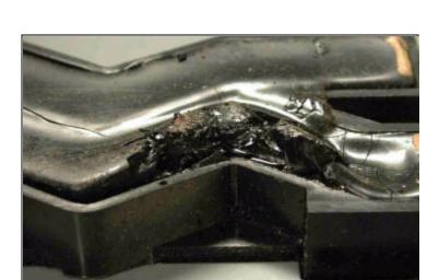
$\underline{FIGURE~3}$  - OVERHEATING AT THE CONTACT BETWEEN THE BUSSBAR AND THE STAB SOCKET ASSEMBLY CAUSED THIS DAMAGE TO THE INSULATION.
