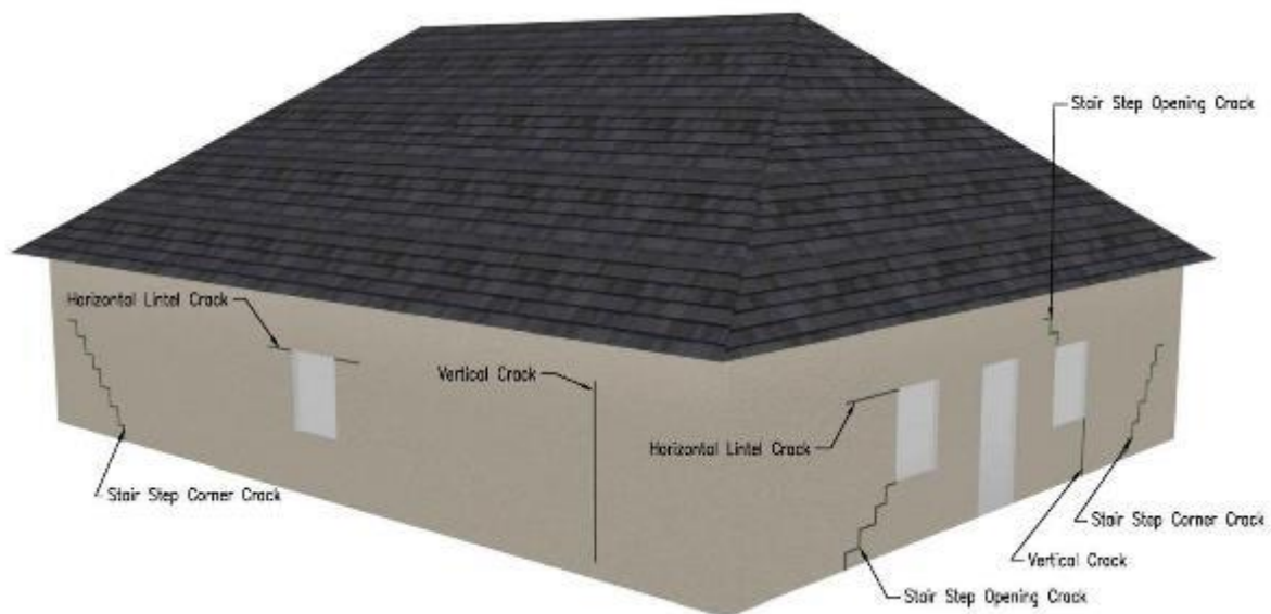
Figure 1 Typical cracks in masonry due to thermal and moisture expansion and contraction.
