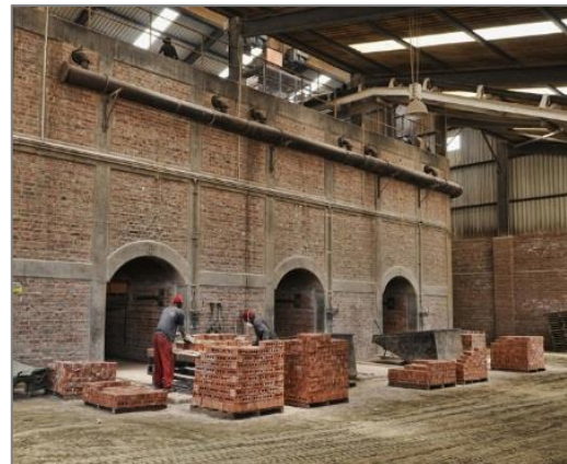
Clay bricks are fired in a kiln at extremely high temperatures. Concrete bricks are dried in the sun.
