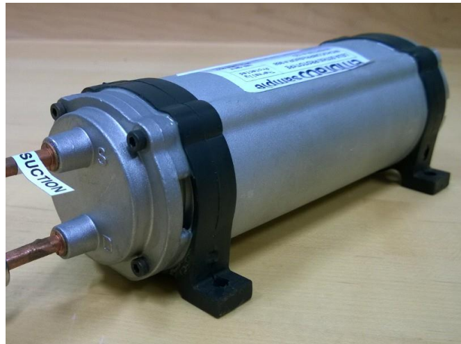
Figure 2.5: 300W Linear Compressor
