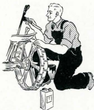
Fig. 52. Brighten rust spots with a wire brush and repaint machinery with rust preventive paint. (See mixing formula, fig. 51.)
