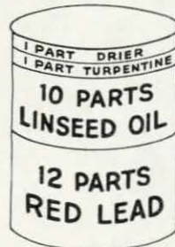
Fig. 51. To paint metal, thin down red lead paste as indicated.
