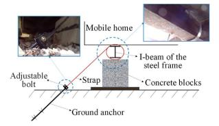
Fig. 1. Standard in-ground anchoring system for manufactured/mobile home.
