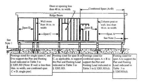
Notes: 1. Bottom of footings must extend below frost line depth, unless designed for placement above the frost line. (See §3285.312(b)).
