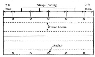
Figure A to § 3285.402 Ground Anchor Locations and Spacing - Plan View.
