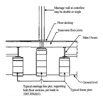
Notes: 1. Mate-line column support piers are installed with the long dimension of the concrete block perpendicular to the rim joists.
