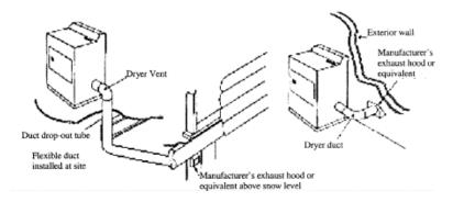
Notes: 1. Installation of the exhaust system must be in accordance with the dryer manufacturer instructions.
