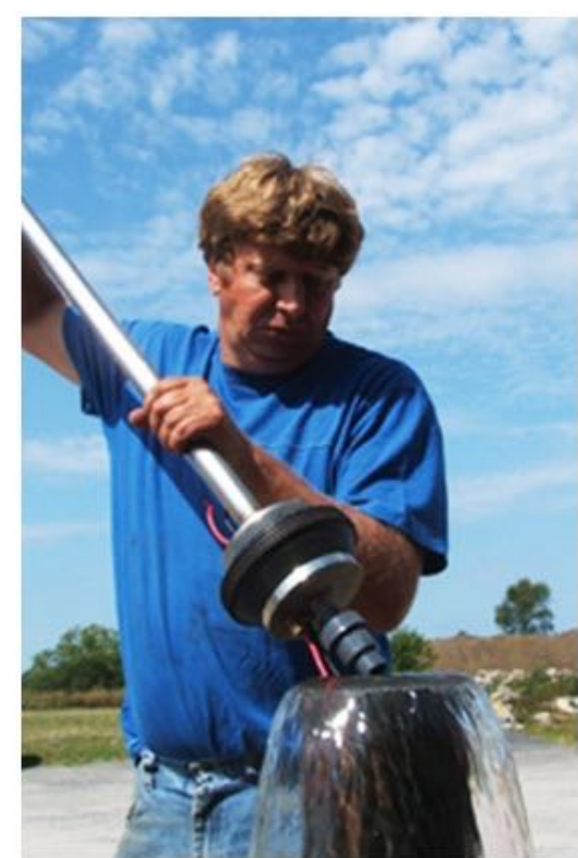
Figure 12-9: Flowing Well Packer
