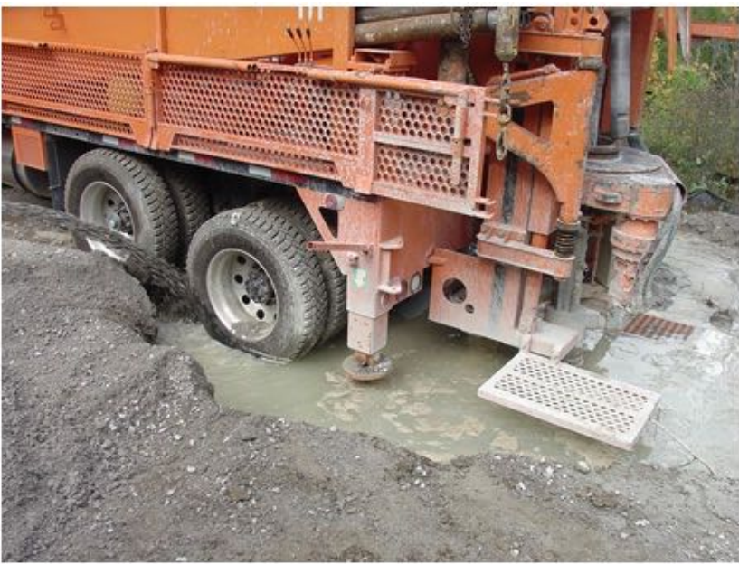
Figure 12-7 shows the same drilling rig and void shown in Figure 12-6. The drilling rig is slowly falling into the hole jeopardizing the drilling rig. In this case, the well contractor took immediate measures to fill the void and rescued the drilling rig.
