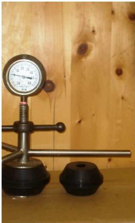
Figure 12-5: Flowing Well Pressure Gauge Device - Installed
