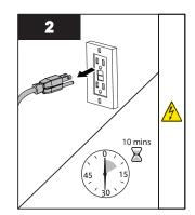
Disconnect main power source and allow the unit to cool for 10 minutes.
