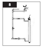
Close the downstream tap once the UV chamber is filled with water, and inspect for any leakages.
