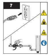
Plug the unit back to the power source. Reset the end of lamp timer alarm back to 365 days.
