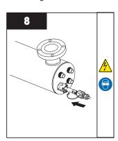
• Connect the lamp connector to the UV lamp.
