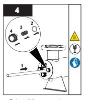
Reinstall the quartz sleeve with lubricated O-rings, followed by spring and retaining nut.
