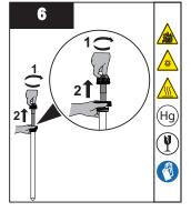
Unscrew the UV lamp by holding the sleeve bolt.
