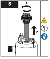
Remove lamp/sleeve assembly along with sleeve bolt from chamber.
