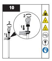
Install and secure the new lamp into sleeve.
