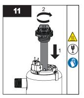
Insert and secure the lamp/ sleeve assembly.
