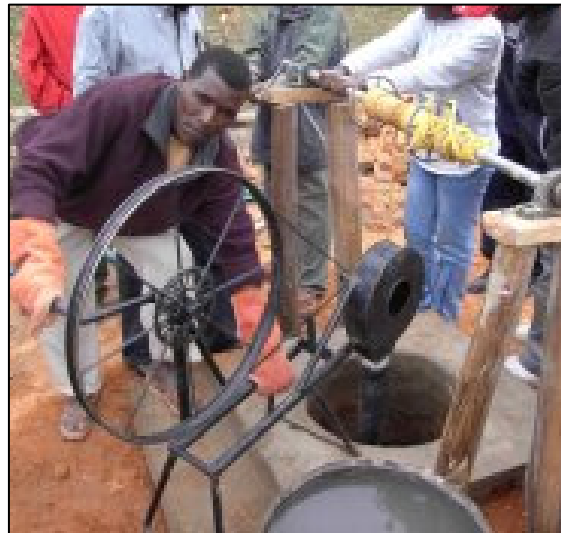
A ventilator for brining fresh air down in the well
