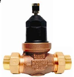
Double threaded end connections to simplify installation with pipe size flexibility. Standard models are equipped with single union end connection O.D. and female NPT threaded end connection I.D. Also available with threaded NPT O.D x NPT I.D. connection on both ends. Several other different end-connection and sizes are available.
