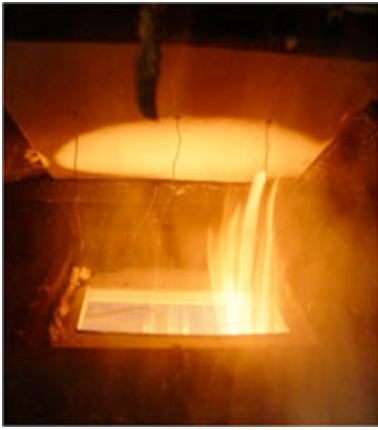
Fire generated by a 150 kw burner on a standard 1/4" vent. Flame and ember penetration within 15 seconds from the start of the fire.
