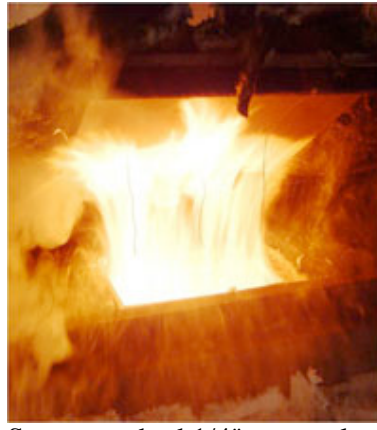
Same standard 1/4" vent only seconds later with enough fire through the vent to engulf the attic and to destroy the home.
