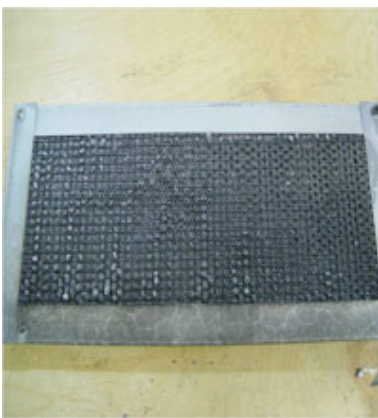
Same Vulcan Vent completely sealed (closed) with no fire penetration into the attic.
