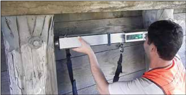
Figure 2.13—Electronic display on a resistance drill.
