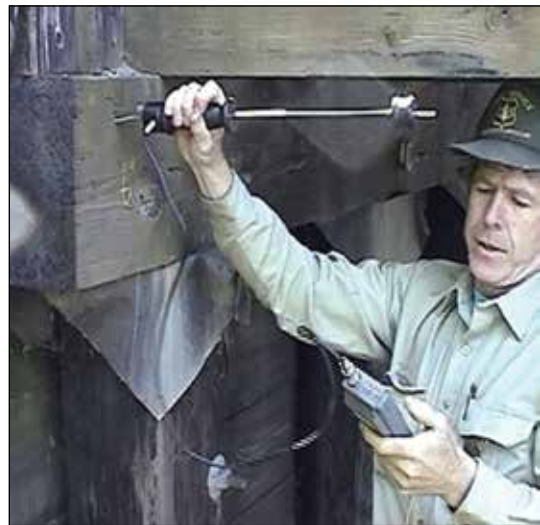
Figure 2.7—A pin-style moisture meter is used to determine moisture content of timber elements.
