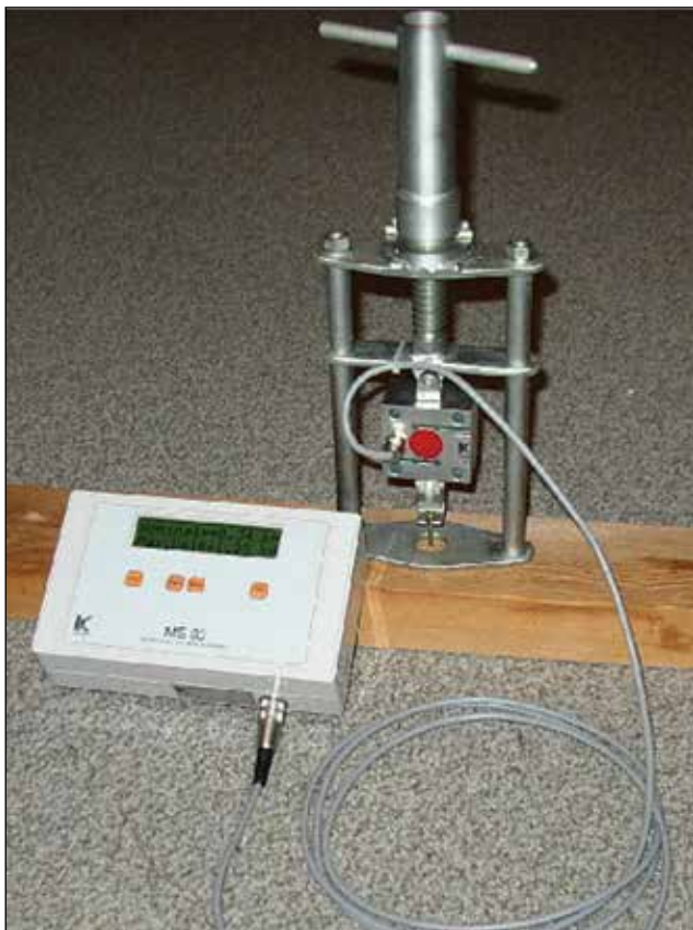
Figure 2.6—Screw withdrawal resistance meter that can be used to assess local wood quality.
