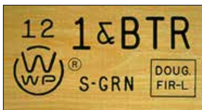
Figure 6.3—Grade stamp from WWSA No. 1 & Better dimension lumber. Moisture content is surfaced green (unseasoned) condition, over 19% (WWPA 2005).
