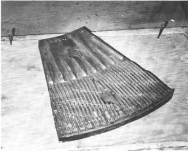
Figure 106—Plate segment of Sprout-Waldron 42-in pressurized refiner.
