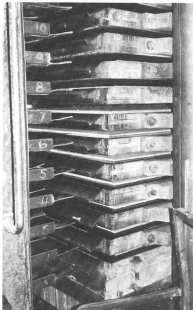
Figure 185 —Loading of S2S press. Mats in position are about 1/2 in thick. Press ready to close.
