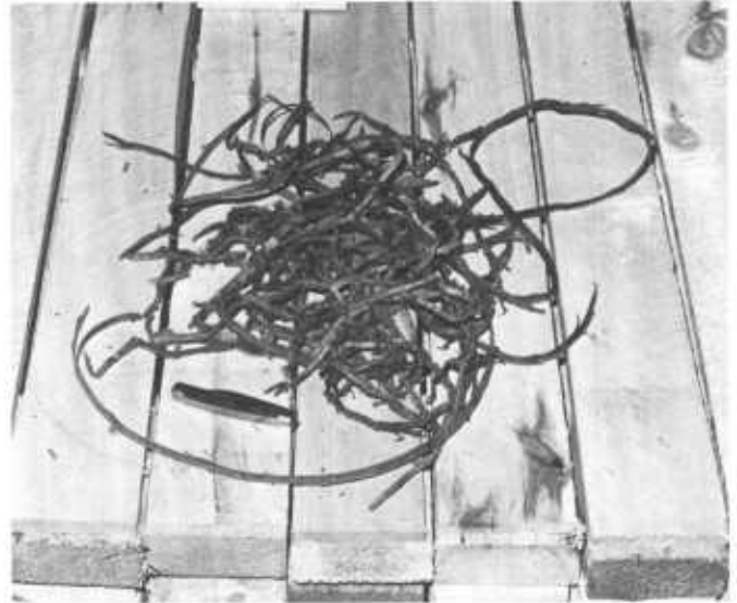
Figure 274 —Shavings generated by fixed panel-scoring knives.
