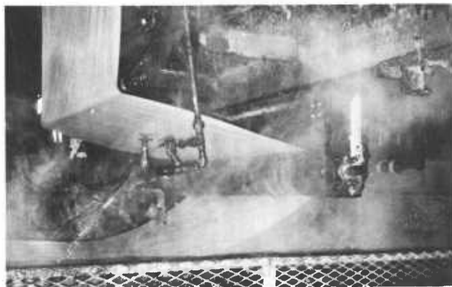
Figure 173—Paper overlay being applied to wet mat.
