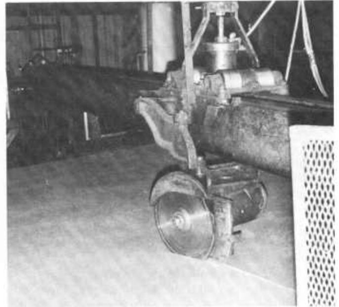
Figure 155—Disk trimmer cutting traveling mat to length. Mat travel is from left to right. Overhead beam travels at same speed and in same direction as mat, while saw travels along beam across mat. When cut is completed the saw lifts up, and beam and saw return to initial position.
