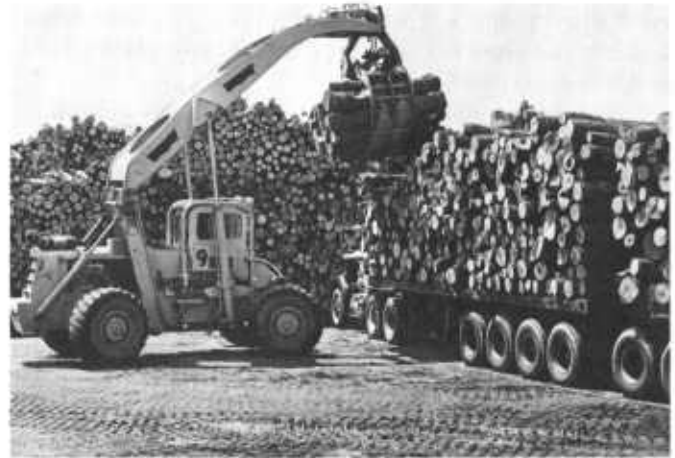
Figure 45—Unloading of truck in woodyard. Total load on truck and trailer approximately 14 cords.
