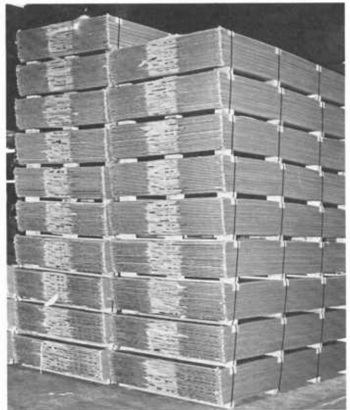
Figure 308 —Wrapped and unitized finished hardboard panels. Panels are wrapped individually. Spacer blocks and wood stringers are included in each package to facilitate handling by fork lift truck.
