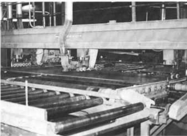
Figure 269 —Outfeed end of cross trimmer. Note feed lugs on infeed side.
