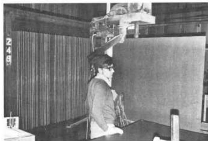
Figure 255—Hardboard being unloaded from buggy and inspected after leaving humidifier. Boards are stacked on edge.
