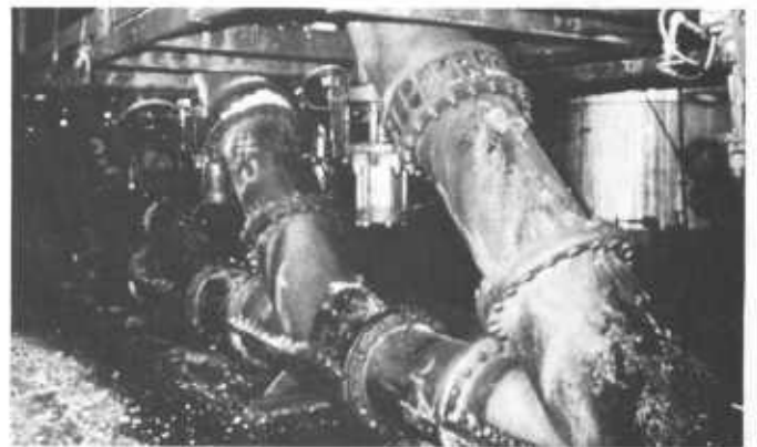
Figure 81 —Discharge tubes of Masonite guns (Masonite Corp.).
