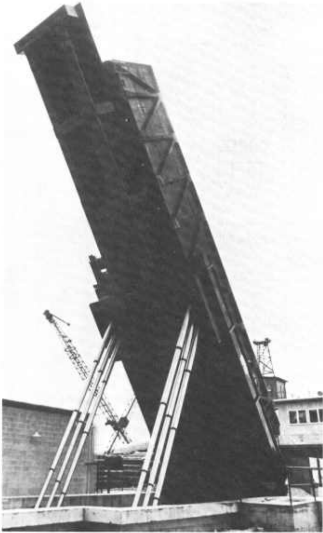
Figure 62—A 300,000-lb-capacity rail car dumper (Peerless).
