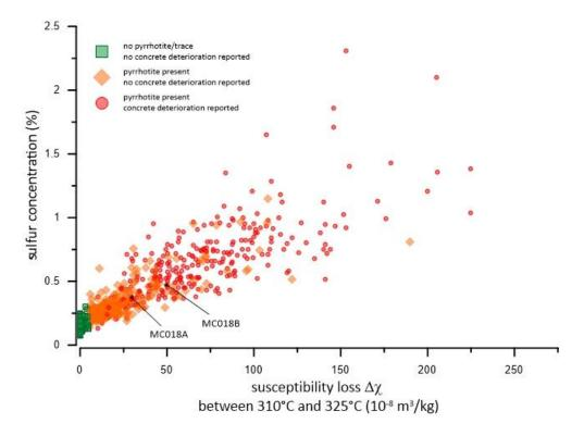
Samples MC018A and MC018B are classified as "pyrrhotite present, concrete deterioration reported" (red circles). We classify concrete as deteriorated due to pyrrhotite if map (spider) cracking is observed or reported on the date of coring. Map cracking was reported on the homeowner's questionnaire (based on engineer's initial visual inspection). To see the details of these results, a second graph is included below and covers a smaller range:
