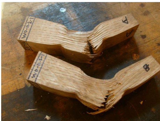
Figure 3-9: Key Bending and Crushing (White Oak Keys)
