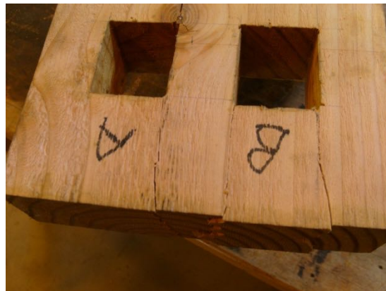
Figure 3-6: Plane Shearing 'A', Relish Failure 'B'
