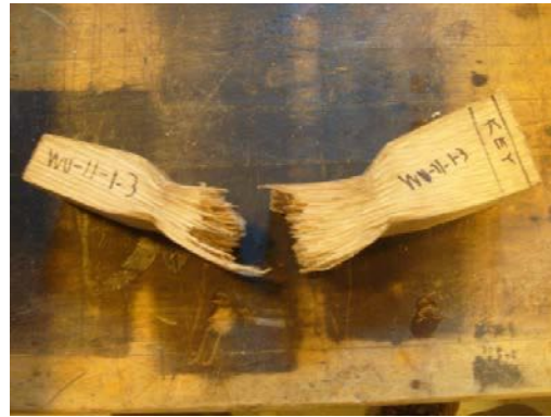
Figure 3-12: Severed Key from Wedging
