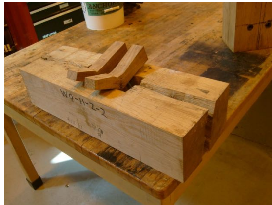
Figure 3-13: Mortise Split from Key Wedging
