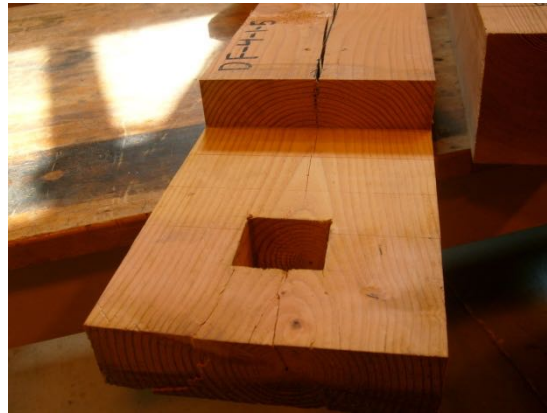
Figure 3-5: Tenon Split (keyhole center)
