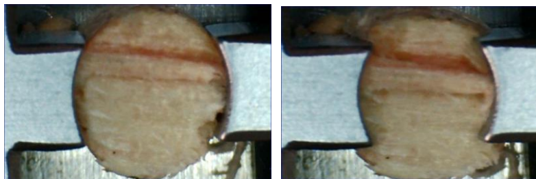
Fig 5a, 5b - Core sample in jaws with force being applied from left and right. Second photo with failure occurring prematurely by shearing as timber grain not in alignment with plane of jaws.
