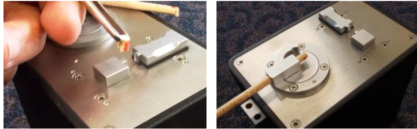
Fig 4a, 4b - Digital Fractometer with 'pellet' being inserted into jaws at left. Optional bending strength feature with timber core being placed at right
