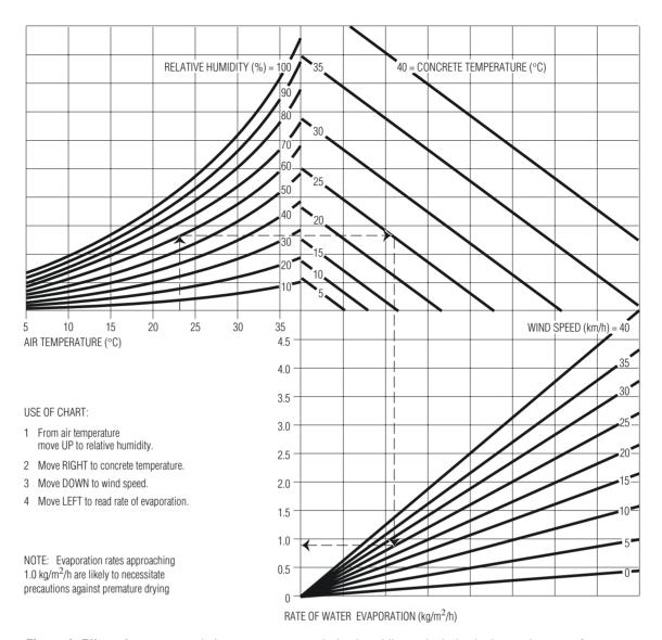
**Figure 1:** Effect of concrete and air temperatures, relative humidity and wind velocity on the rate of evaporation of surface moisture from concrete (after ACI 305<sup>2</sup>)
