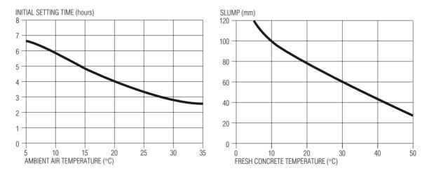
**Figure 2:** Influence of air temperature on setting times of concrete made with Type GP cement
