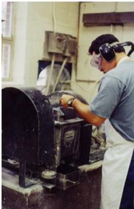
Figure 3.4 samples crushed in mechanical crusher
