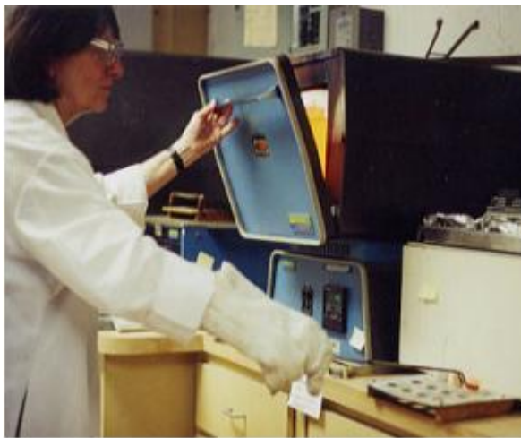
Figure 3.6 Samples removed after ignition at 1832^\circ\text{F} .
