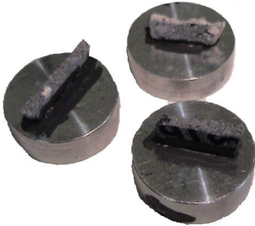
Figure 3.14. Mortar samples mounted on stubs for SEM examination
