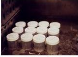
Figure 3.3 Samples cured in four-ounce polypropylene jars after demolding
