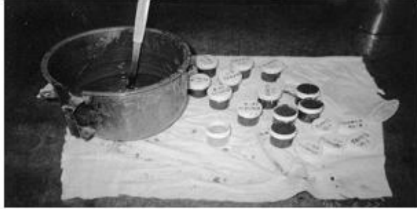
Figure. 3.1 Paste samples cast in one-ounce polypropylene screw cap jars.
