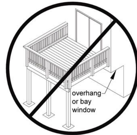
Figure 18. No Attachment to House Overhang
