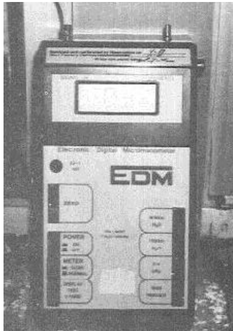
Above: A smoke tube, which is one type of chemical smoke device. Used to observe patterns of air movement and the direction (negative or positive) of pressure differences. Below: A microman-ometer. Used for measuring pressure differentials to learn about airflow. Provides quantitative data, as compared to the qualitative information provided by chemical smoke.
