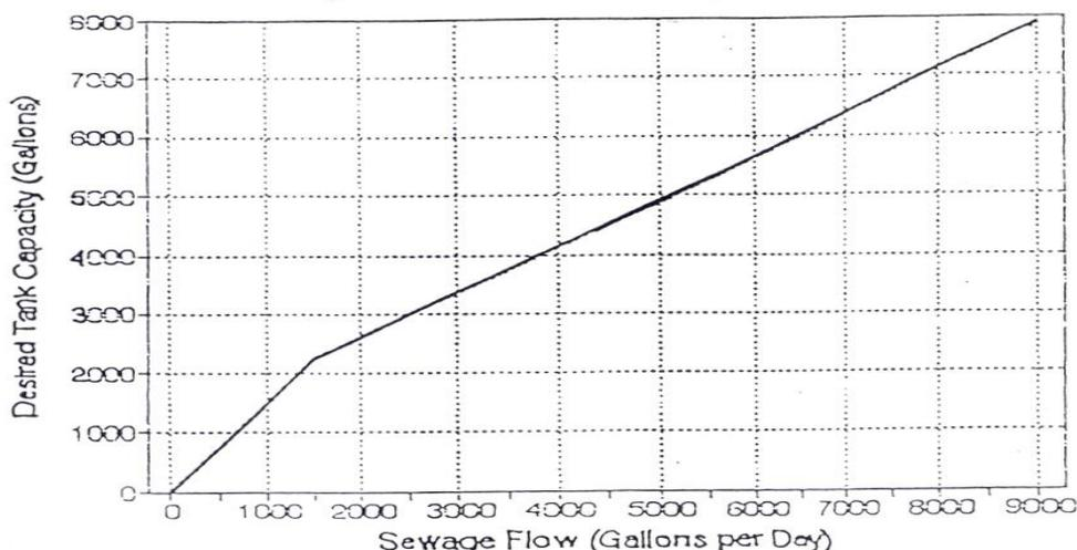
**RESTAURANTS:** *To provide cooling of dishwasher wastes for grease coagulation, provide twice the capacity shown on graph.*
