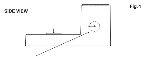
**NOTE**: The bottom of the additional fixture 3" diameter hole must be 5" minimum above the base of the tank as shown. Cut out spotting template below. Pipe installed in this 2" seal must be supported vertically.
