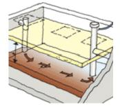
The partially decomposed solids that settle on the bottom of the tank must be pumped out approximately every 3-5 years, depending on use.
