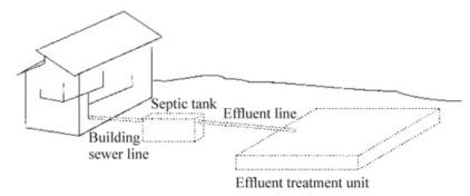
Figure 1. Typical components of an onsite wastewater treatment system.
