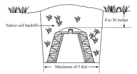
Figure 3. Gravelless trench with slotted sidewall chamber.
