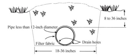
Figure 2. Gravelless trench with pipe and filter fabric.
