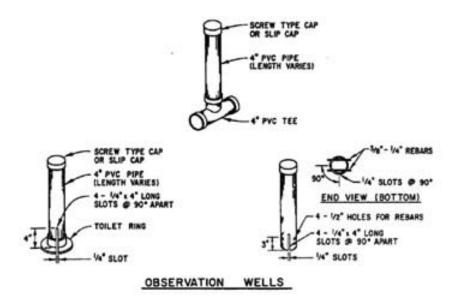
Figure 3.16 Support options for monitoring tubes.
