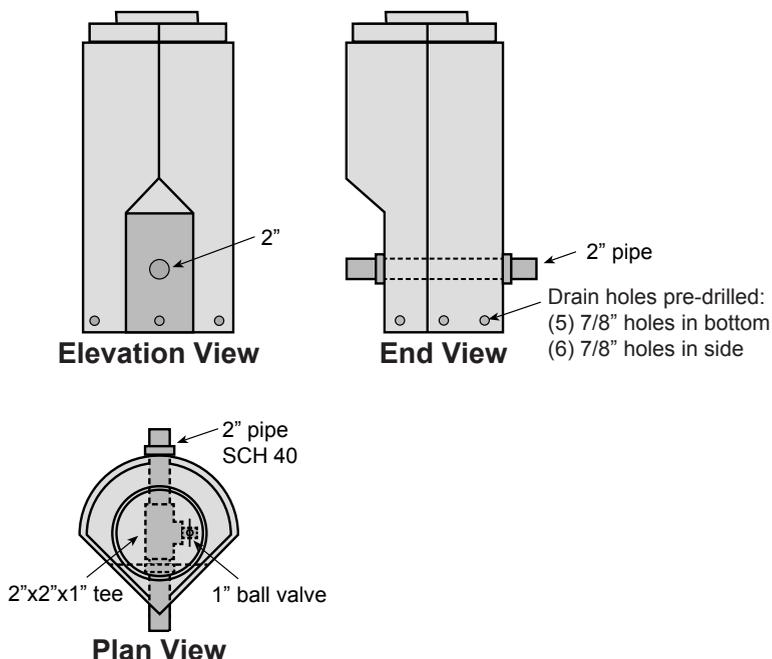
**Typical Configuration Puraflo Dn Type A – Pad**
