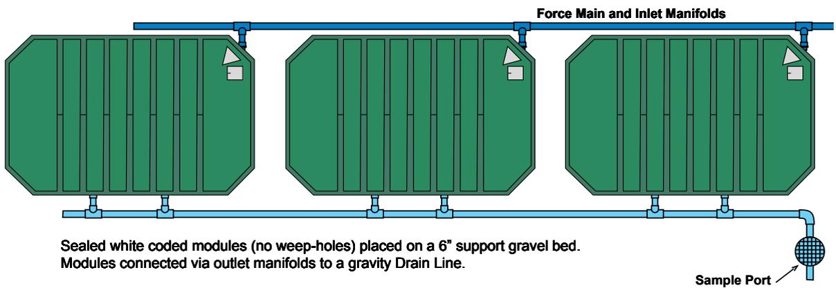
Sealed white coded modules (no weep-holes) placed on a 6" support gravel bed. Modules connected via outlet manifolds to a gravity Drain Line.
