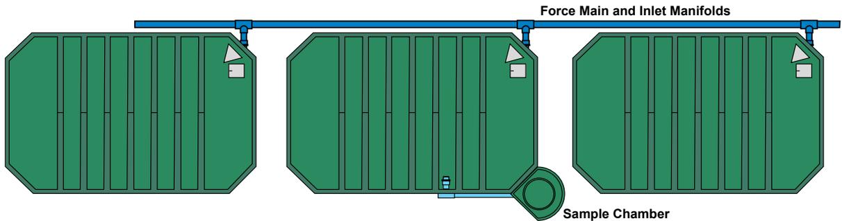
Blue coded modules with weep holes and one green coded module with sampling chamber, drain into a stone pad for final treated effluent disposal. Pad dimensions can be selected to match site conditions and modules can be installed side-by-side as well as end-to-end (as shown above)
