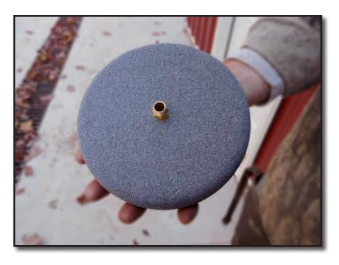
The airstone is a hard stone-like disc that have fine holes all through it. As the air passes through the stone, the air breaks down into a fine mist of air bubbles. As the bubbles rise to the surface, some of the oxygen on the air will be trapped in the water. Also, the windmill will keep a circle of water open even in the coldest part of winter, therefore providing a place for ducks to swim and protect themselves from predators.
