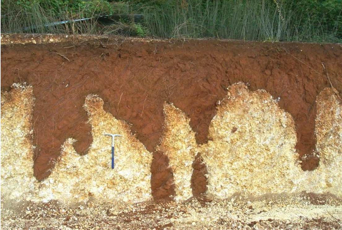
Figure 6.4: Typical limestone / soil interface. 6-inch percolation test pits just a foot or two apart can give very different percolation rates. (Photo courtesy Bob Gavenda, NRCS)
