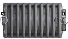
3b. Assemble all Arc chambers in the trench excavation by first placing the "dome end" of the incoming chamber over the "post end" (B) of the chamber already in place. Raise the post end of the incoming chamber and slightly pull the chamber back until the dome stops and is locked into the post end joint.
