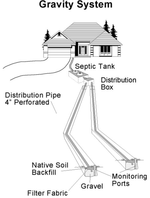
Virtually all OSSs use a septic tank to separate the oils and solid components of sewage from the wastewater. The oils and solids are retained in the tank, while the wastewater "effluent" flows into a drainfield or more complex wastewater treatment device. In a
