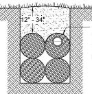
COVER EZFOW BUNDLES WITH UNTREATED BUILDING PAPER, 2-INCH STRAW LAYER, OR OTHER APPROVED BARRIER MATERIALS IF NOT USING A GEO PRODUCT
