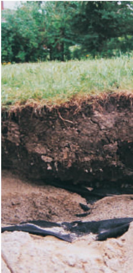
Failure of this system was due to the use of clay as the back-fill material over the geotextile.
