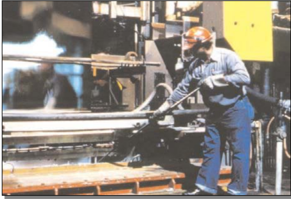
Figure 3-6 Zinc Coating of Steel
