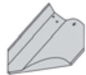
Figure 40.2 Spanish Cut and Closed Valley Tile
