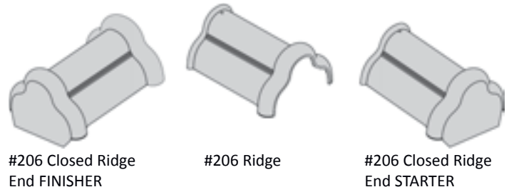
Figure 46.2 Ridge Starter Finisher Diagram
