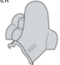
Figure 46.6 102/206 1 Hip/2 Ridge Terminal
