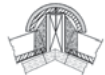
Figure 41.3 Mortared Hip Detail
