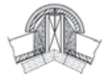
Figure 53.3 Mortared Hip Detail
