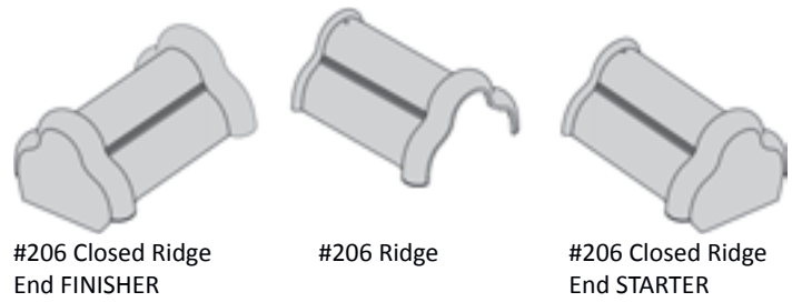
Figure 46.2 Ridge Starter Finisher Diagram
