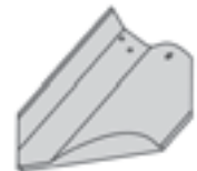
Figure 40.2 Spanish Cut and Closed Valley Tile
