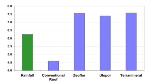
Illustration 5: pH (median) of the runoff from the tested substrates between 8/7/97 and 1/21/98
