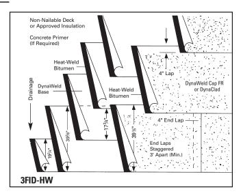
Heat Weld a full width piece of one of the cap sheets listed over the installed base felt. Subsequent sheets are to be applied in the same manner, with 4" (102 mm) side laps and 4" (102 mm) end laps over the preceding sheet.
