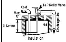
"Alternate" Only when the tappings are not provided Use Standard or extra length extension thermostat.
