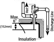
Vertical discharge line must be installed with its direction downward.
