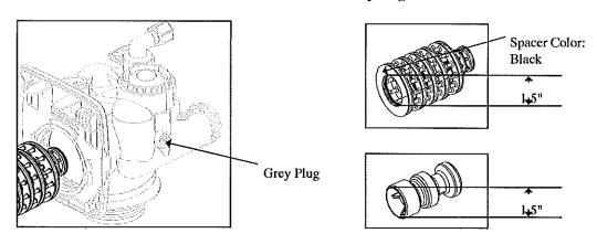
WS1.25 with 32mm Distributor Tube Opening Identification
