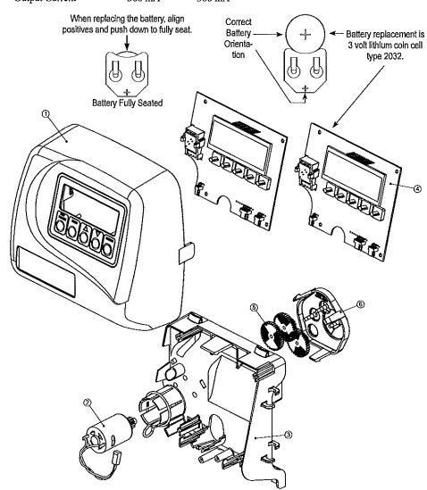
WS1 Drive Cap Assembly, Downflow Piston, Upflow Piston, Regenerant Piston and Spacer Stack Assembly
