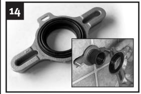
Place the seal into the flange with the ribs facing out. Install the flange with washers and hex nuts, but do not tighten completely.
