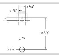
Carrier stud placement: If using inwall carrier, set bearing rods as shown
