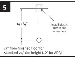
If in-wall carrier is not used, measure and mark the rough-in. Use a 5/16 masonry bit to drill hole, then install the hanger bracket with one plastic anchor and screw.
