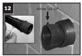
Apply lubricant to the outside of the rubber bushing and ribbed inside area. Insert the tube and bushing with the arrow tab at the top.
