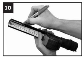
Find the drain nipple depth on the cutting chart (left) and mark the specified trim length on the insert tube at the nearest 1/4" groove.
