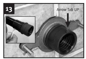
Apply lubricant to the outside of the rubber bushing and ribbed inside area. Insert the tube and bushing with the arrow tab at the top. Lube tailpipe of housing.
