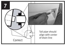
Re-hang and re-check bowl alignment with the drain line. Mark anchor holes then remove the bowl without moving the hanger bracket.
