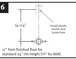
a 5/16" masonry bit to drill hole, then install the hanger bracket with one plastic anchor and screw.
