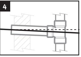
If standing water is present, adjust drain to achieve pitch (code requires 1/4" drop per foot of drain line for proper pitch). Seal the wall according to code.
