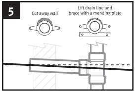
If standing water is present, adjust drain Measure and mark the rough-in. Use to achieve pitch (code requires 1/4" drop per foot of drain line for proper pitch). Seal wall according to code.
