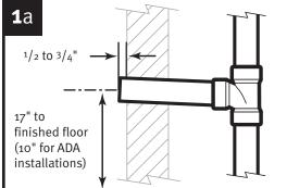
Set drain line height at 17" from finished floor (standard 24" rim) or 10" for ADA installation. Threaded nipple should extend  $\frac{1}{2}$  to  $\frac{3}{4}$ " from wall.
