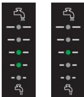
Fig. 13 SCALA2 outlet pressure indication
