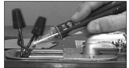
Figure 32 - Non-Contact Circuit Tester
