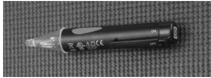
Figure 28 - Non-Contact Circuit Tester
