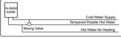
For Space Heating Purposes: If the system requires water for space heating at a higher temperature than for other uses, means such as a mixing valve shall be provided to temper the water for the other uses to help prevent scalding.
