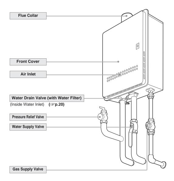
\* The above illustration shows an example of installation. The exact installation configuration may be slightly different.
