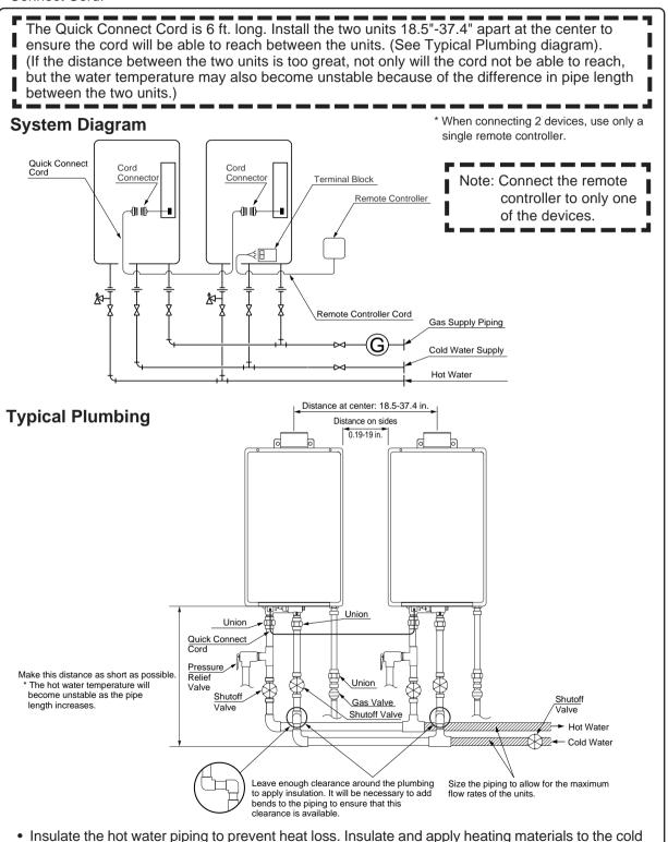
water supply piping to prevent heat loss and freezing of pipes when exposed to excessively cold
