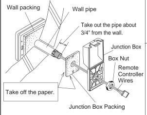
Connect the remote controller wires to the separate remote controller cord inside the box.
