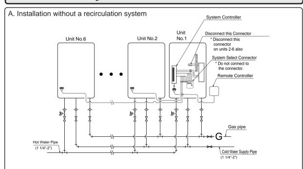
• Insulate or apply heating materials to both the cold water supply piping and the hot water piping to prevent freezing during cold weather and to prevent heat loss through the piping.
