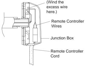
Tie the redundant length of the remote controller cord outside the junction box.
