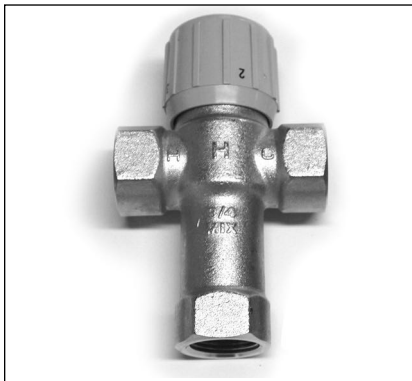
Figure 7 - Thermostatic Mixing Valves installed at each point-of-use can help prevent scalding. Install Thermostatic Mixing Valves (figure 7) to regulate the temperature of the water supplied to each point-of-use (for example, kitchen sink, bathroom sink, bath, shower). Consult the valve manufacturer's instructions or a qualified person.
