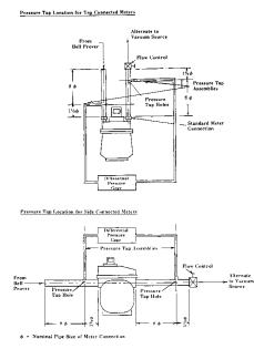
Figure 5. Large Meter Test Apparatus
