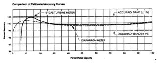
Figure 6. Diaphragm Meter Accuracy
