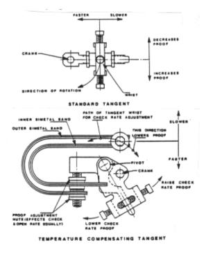
**Figure 3. Tangent Adjustments**
