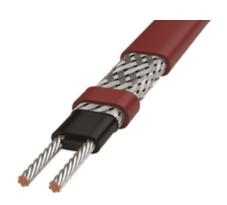
nVent RAYCHEM HTV self-regulating heating cable is designed for freeze protection or process temperature maintenance of pipes and vessels up to 205°C continuously, with a maximum exposure temperature of 260°C. The HTV cable has a solid construction with a high power retention (HPR) heating core and pressure extruded electrical insulation. It is then integrated with a robust metallic braid and a chemically resistant fluoropolymer outer jacket.
