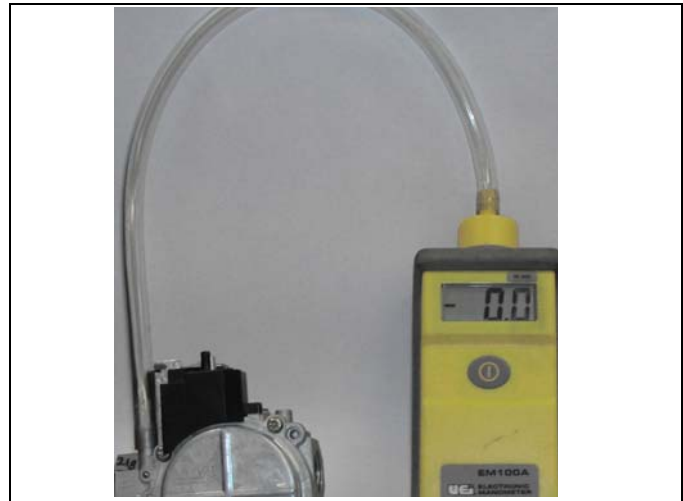
FIGURE 6: Tube Over Inlet Test Port Housing
